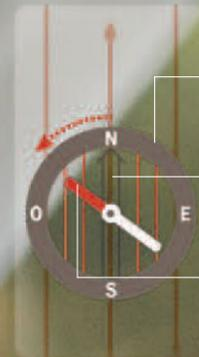
2 The graduated dial is rotated until the pointer is lined up with the magnetic needle.
