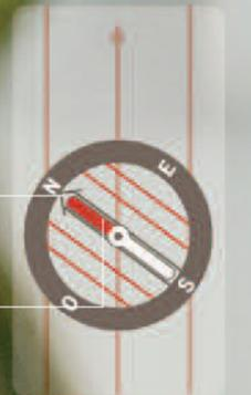
3 Keeping the pointer lined up with the needle ensures that the direction is maintained.
