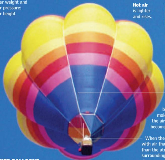
A propane gas burner heats up the air inside the balloon. As the air molecules are heated, the air expands and becomes less dense.
