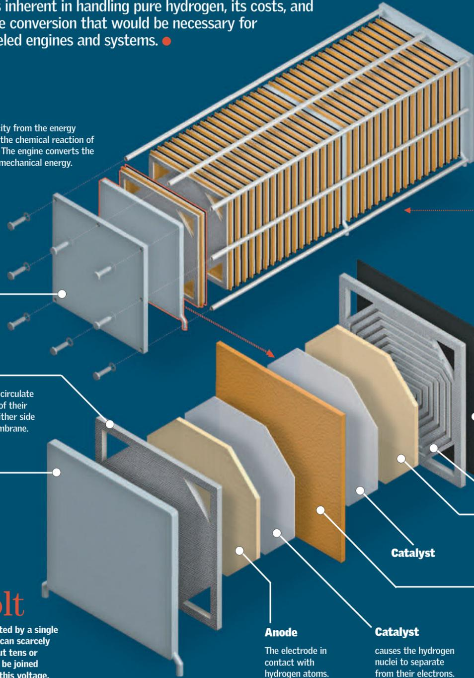
**200** is the average number of hydrogen cells a car engine needs.
