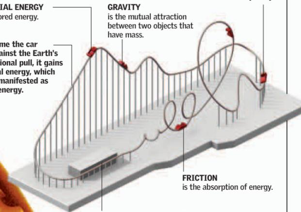
The friction of the wheels against the rails results in the loss of potential energy, causing the train to eventually stop.
