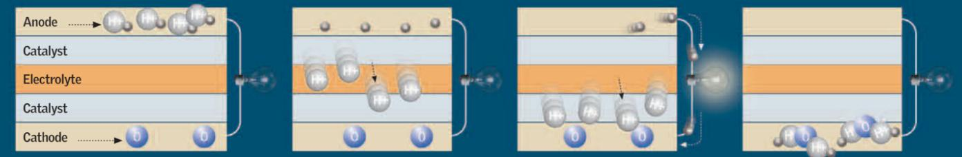
**1** Hydrogen collects at the anode and oxygen at the cathode. The catalyst separates the hydrogen electrons from their nuclei.
