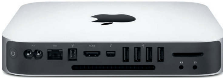
Figure 2-6: The Mac mini's back, showing cable connections.
