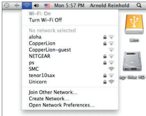
Figure 9-4: You have lots of Wi-Fi networks to choose among, including two that are open.
