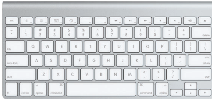
Figure 3-4: Apple wireless keyboard. Note the row of smaller function keys along the top.
