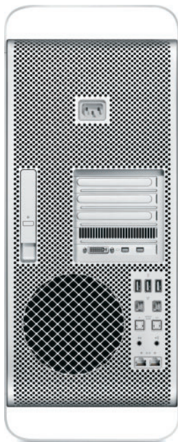
Figure 2-9: Mac Pro from the back, showing slots and cable connections.
