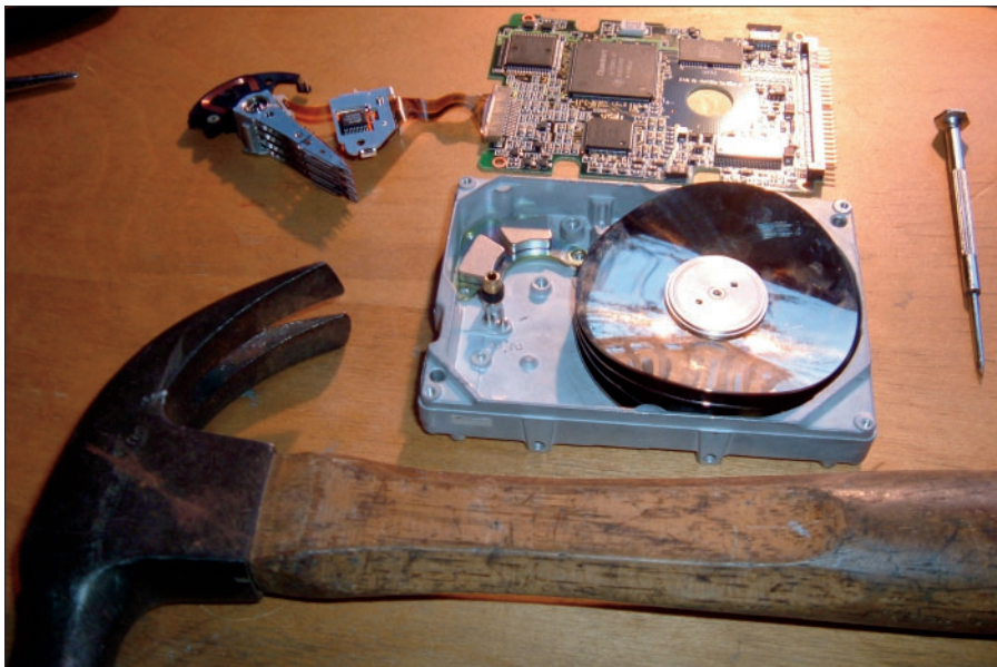
Figure 6-2: Dis- assembled hard drive with bent disks.
