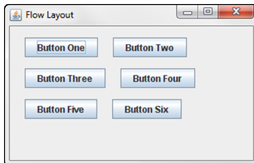
Figure 5-2: Flow layout with left alignment and gaps.
