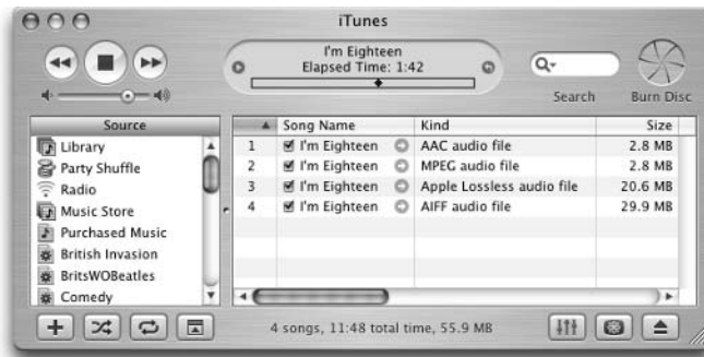
Figure 13-2: Compare the file size of the same song saved in four different file formats.
