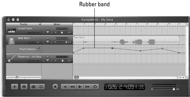
Figure 4-10: This rubber band tells the track “Fade in, play a few seconds, get softer, get louder, and fade out.”
