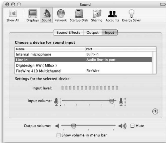
Figure 8-1: Choose the input your guitar is plugged into; don't choose Internal microphone or your ears will get a nasty surprise.
