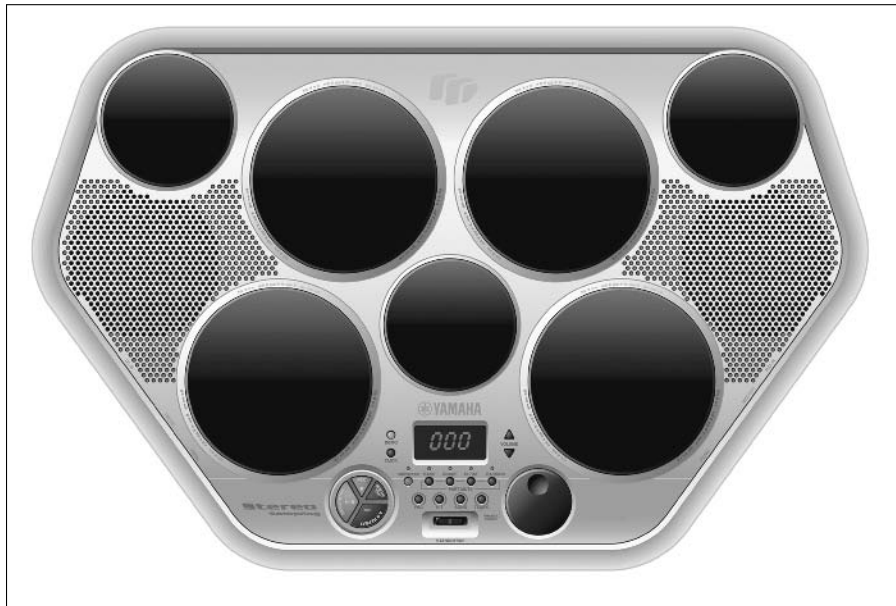
Figure 7-3: Yamaha's DD55 looks, feels, and sounds like real drums, and sends touch-sensitive MIDI information to your Mac.
