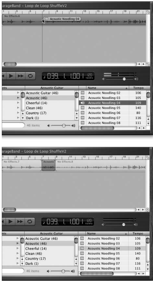
Figure 5-9: Dragging a loop onto an existing track (top) erases the part of the track that it replaces (bottom).
