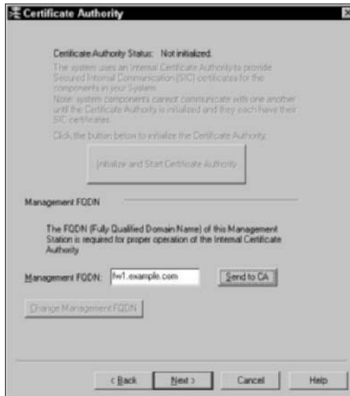
Figure 17-8: Defining the manage- ment station FQDN.
