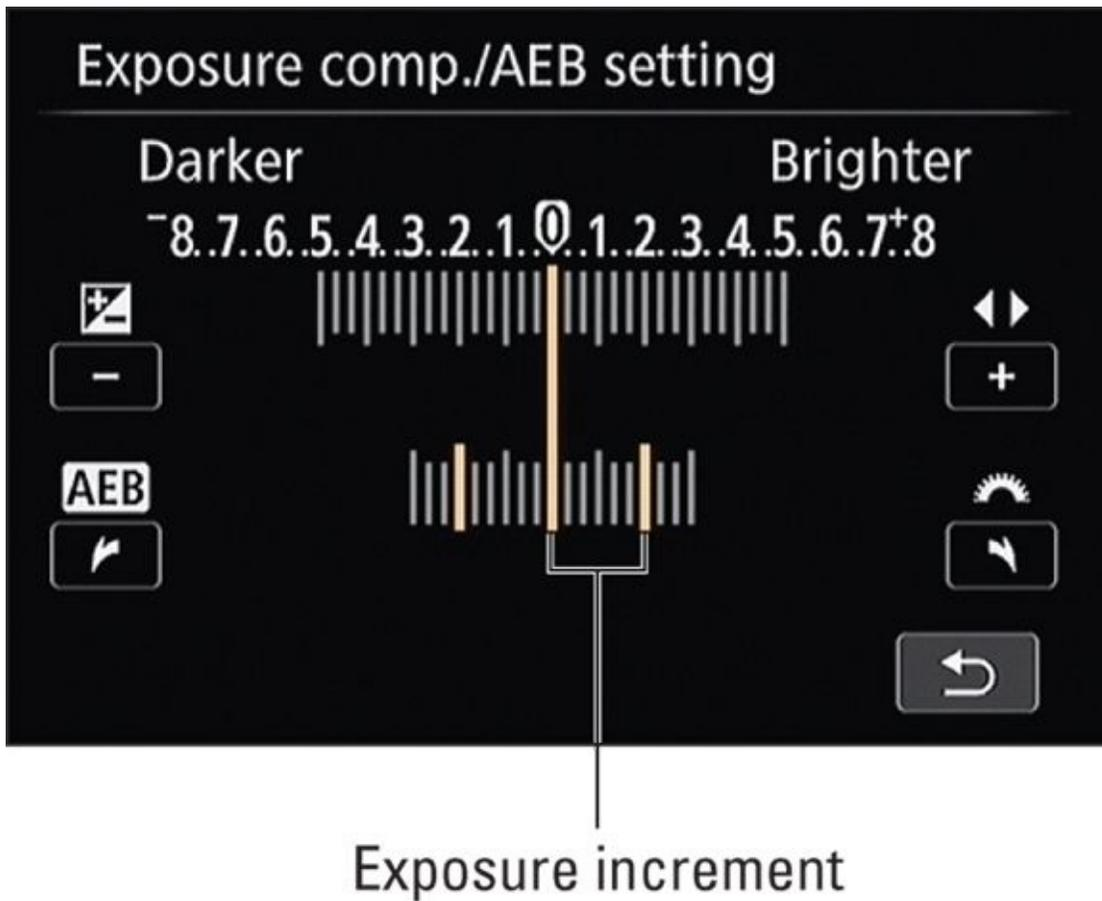
**FIGURE 6-4:** Setting the EV difference between brackets.
