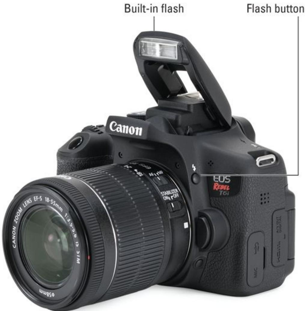
**FIGURE 2-1:** The pop-up flash extends above the camera, ready for action.
