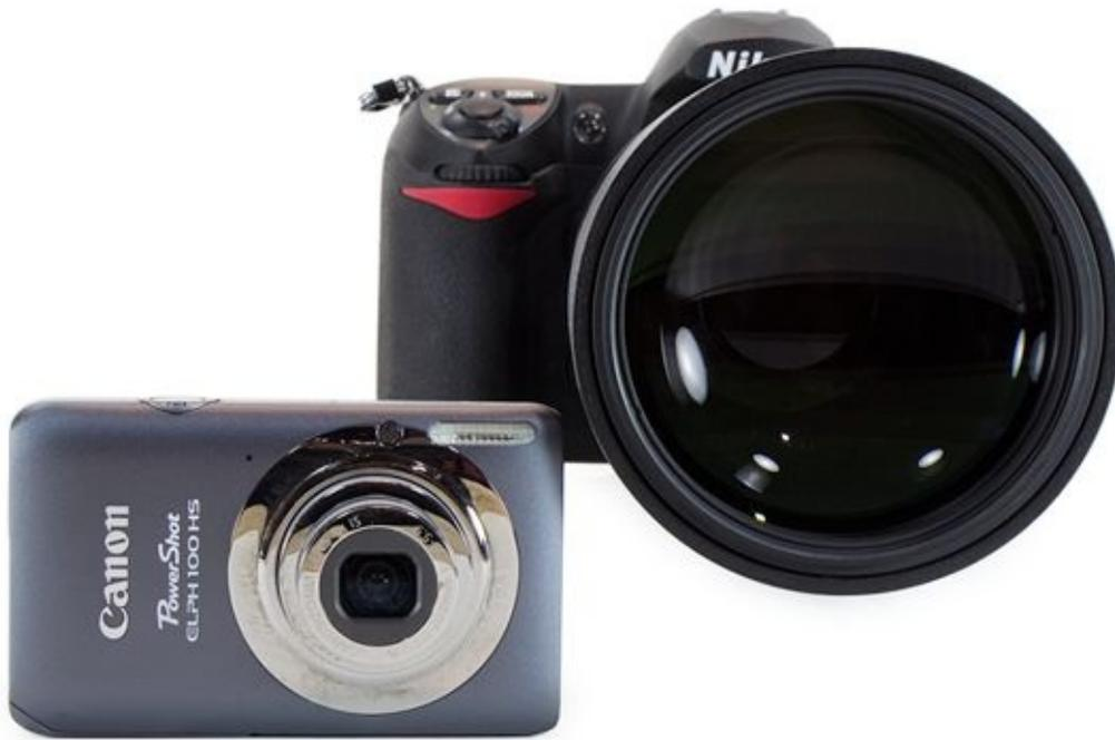
**FIGURE 1-26:** The ability to change lenses is a strength of the dSLR over a compact camera.
