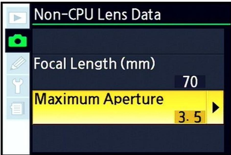
**FIGURE 2-5:** Setting non-CPU lens data in the camera.
