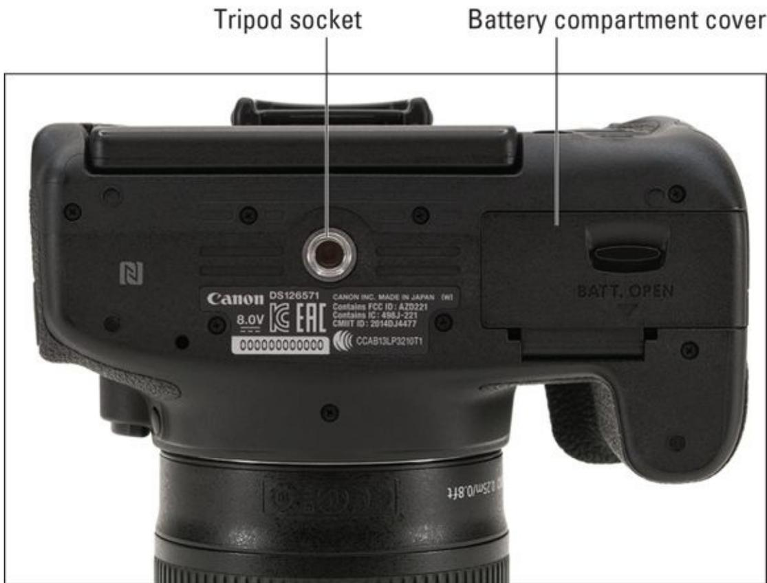
**FIGURE 2-4:** The bottom of a typical dSLR.
