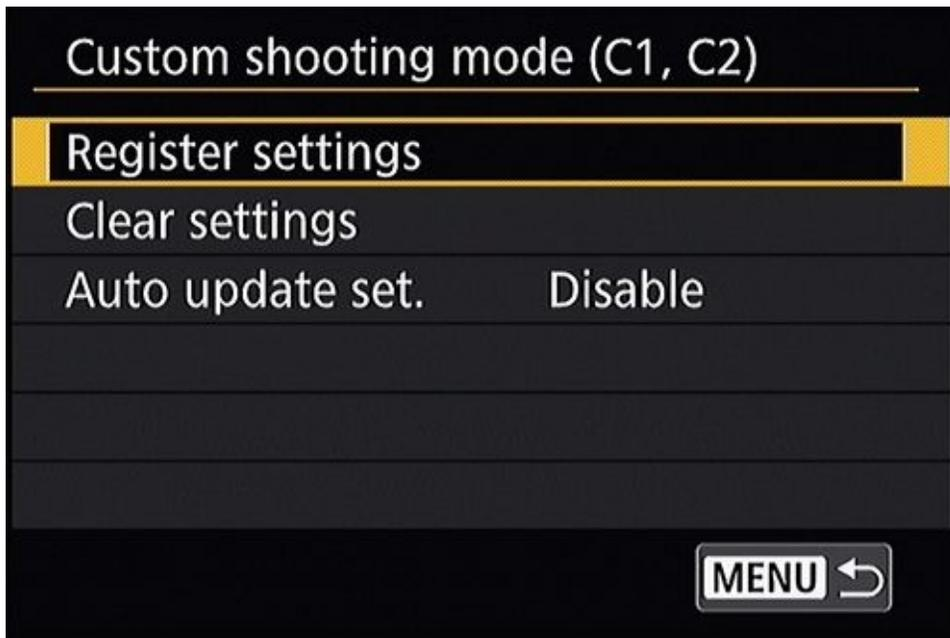
**FIGURE 4-27:** Customize the camera by saving your settings into a special mode.
