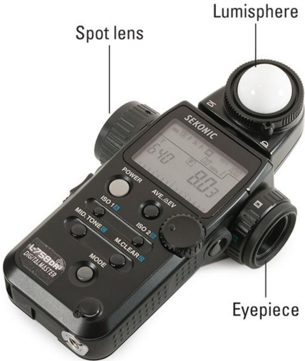
**FIGURE 1-12:** This Sekonic light meter is ready for action.
