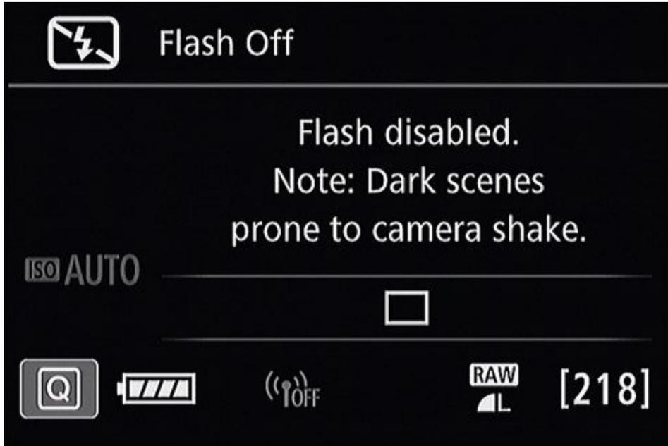
**FIGURE 2-3:** Flash Off mode is an automatic mode that disables the flash.
