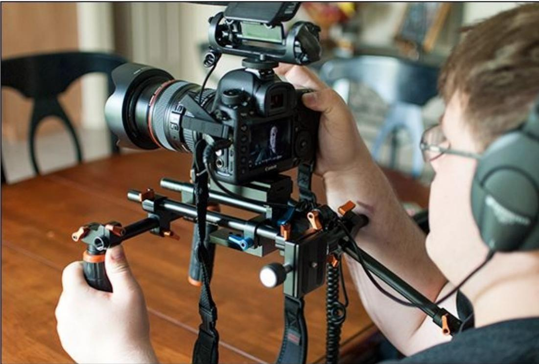
**FIGURE 1-13:** Shooting a video with a professional Canon dSLR and extensive rig.
