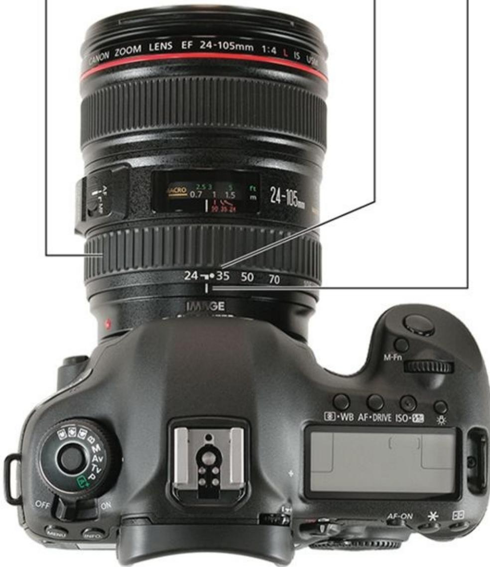
**FIGURE 3-20:** Zoom lenses have a focal length scale on top.
