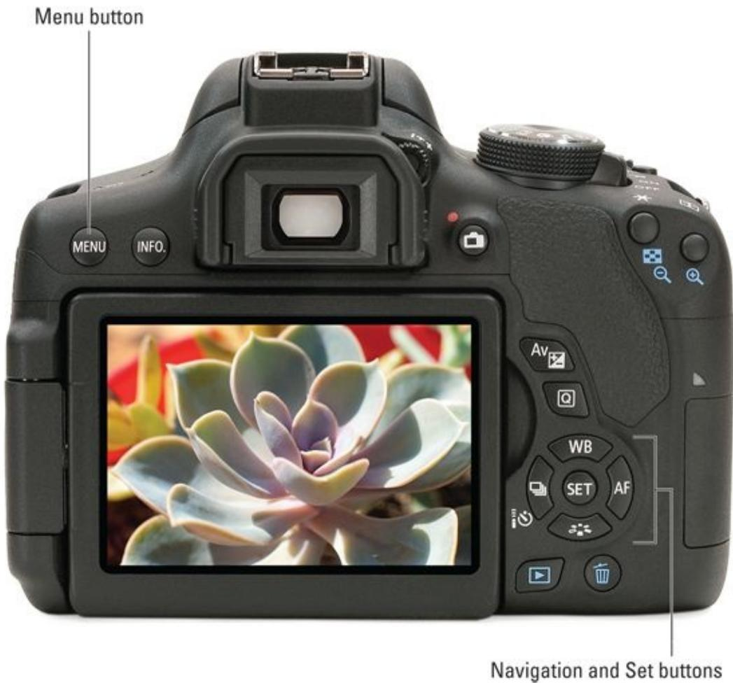
**FIGURE 4-1:** This camera's Menu button is very conveniently placed.
