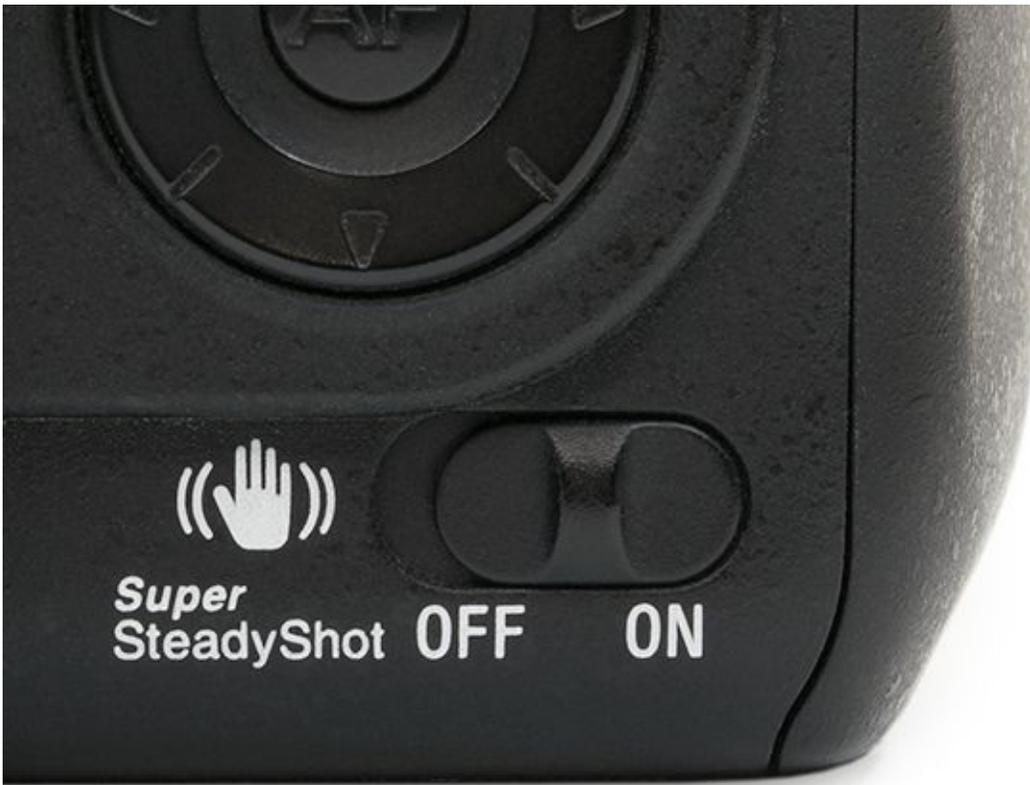
**FIGURE 1-19:** This camera features in-body image stabilization, complete with an on/off switch.
