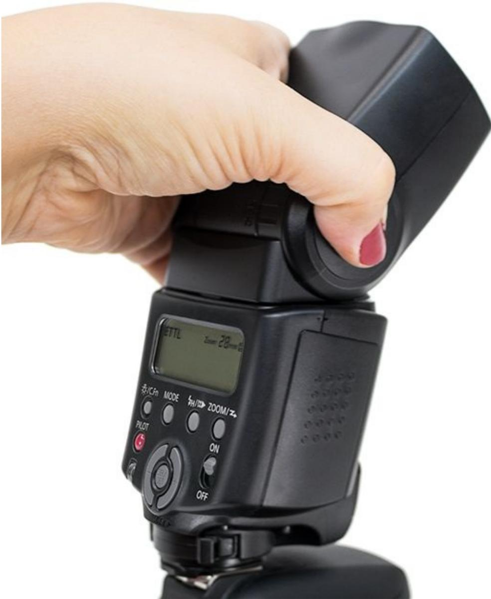
**FIGURE 3-6:** Make sure to hold the lock-release button as you tilt and swivel the head.
