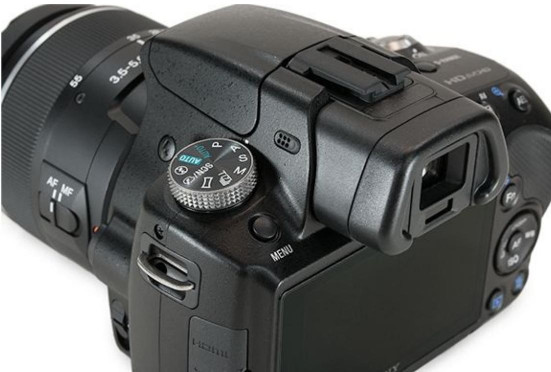
**FIGURE 1-5:** Whether optical or electrical, the viewfinder enables you to see through the lens.
