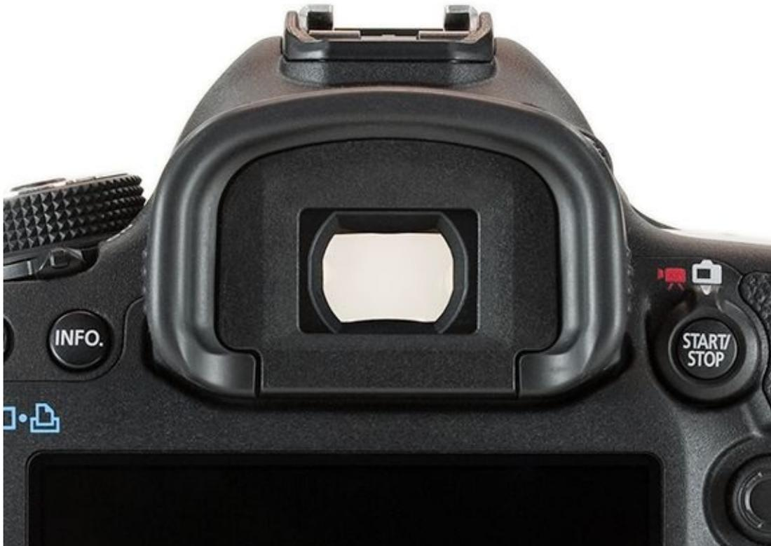
**FIGURE 1-17:** This camera has a nice, large viewfinder with 100 percent coverage.
