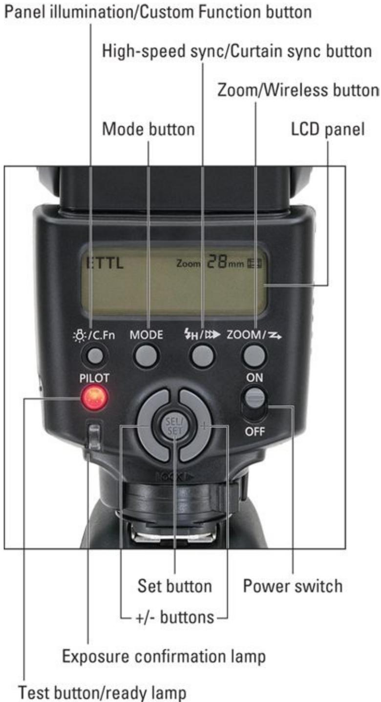
**FIGURE 3-7:** These controls are common to most external flash units.
