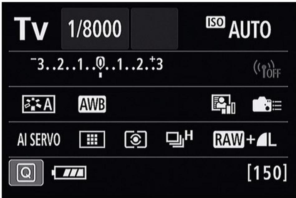
**FIGURE 1-11:** This camera has a maximum shutter speed of 1/8000 second.
