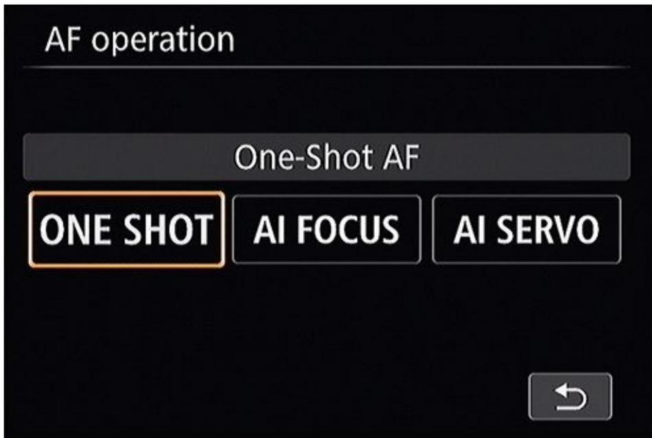
**FIGURE 5-21:** This mode determines whether or not the camera keeps autofocusing.
