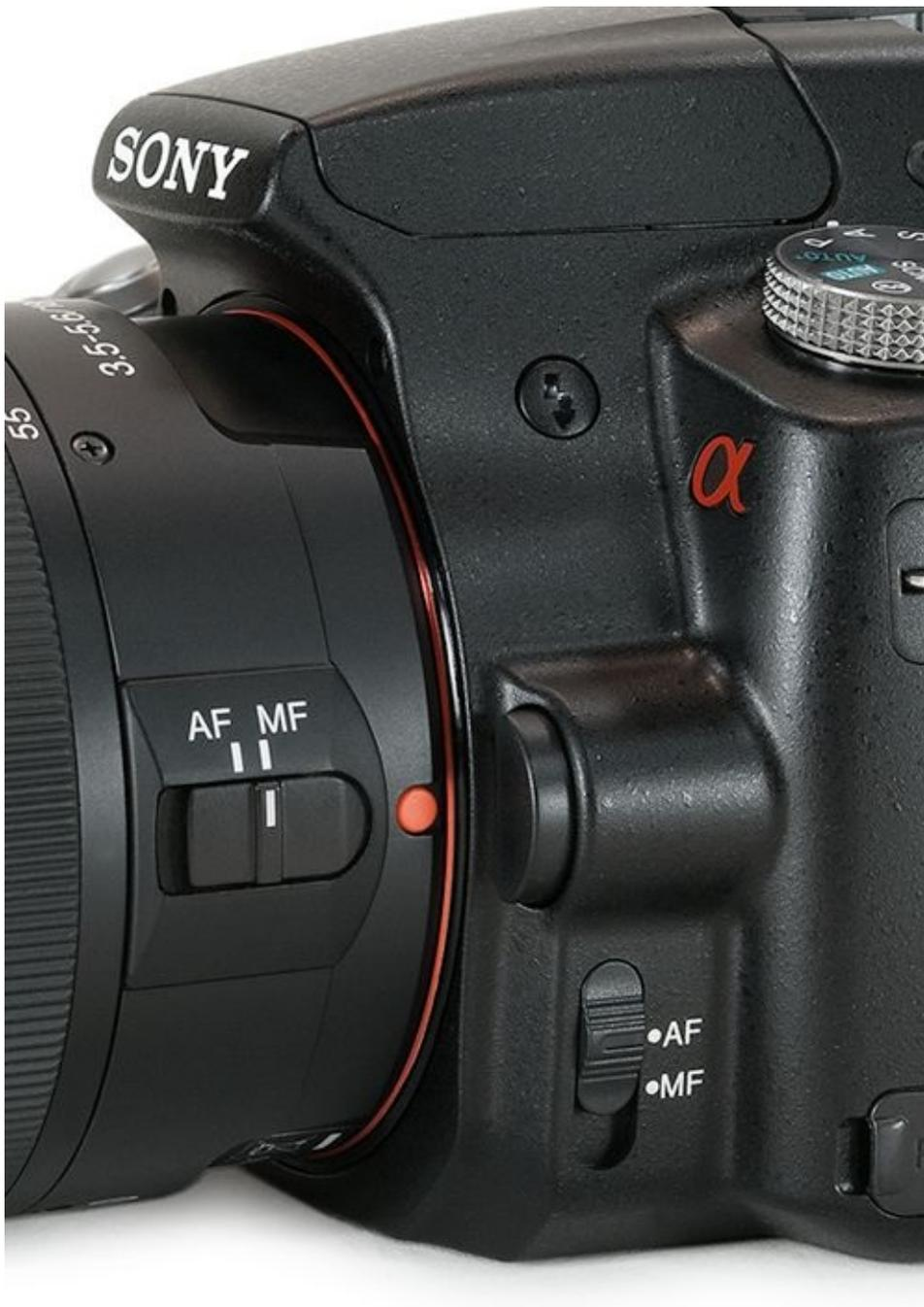
**FIGURE 3-22:** Switch to MF to take total focusing control.
