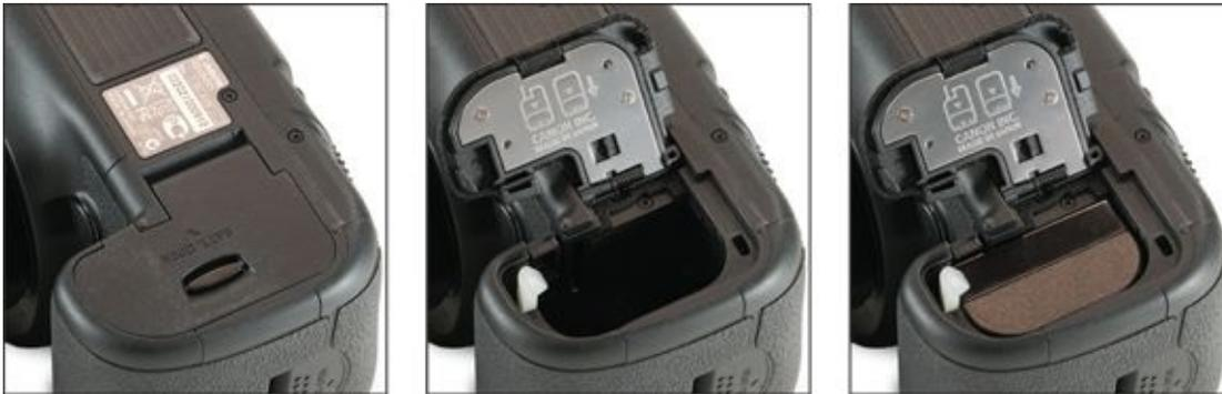
**FIGURE 2-17:** Be sure to move the locking lever out of the way as you insert the battery.
