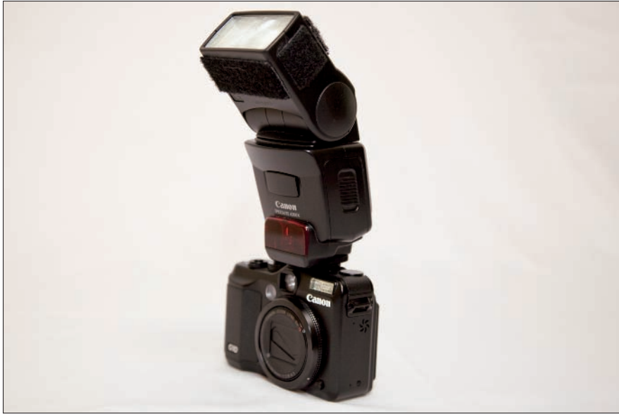
Figure 7-3: A flash with a swivel head can be used to bounce the flash.
