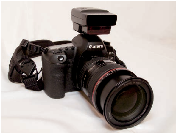
Figure 7-17: Using a wireless transmitter to trigger off-camera flash units.
