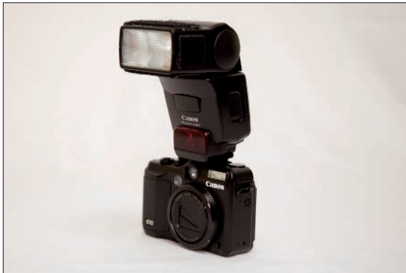
Figure 7-1: Mounting an auxiliary flash unit in the camera hot shoe.
