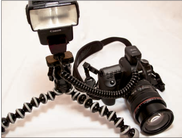
Figure 7-16: Using a hot shoe cord to connect the flash to the camera.
