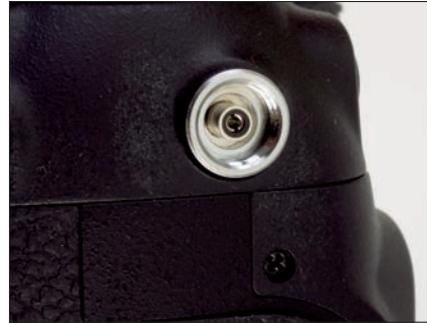
**Figure 2-6:** Your camera may have a connection for plugging in an external flash unit.
