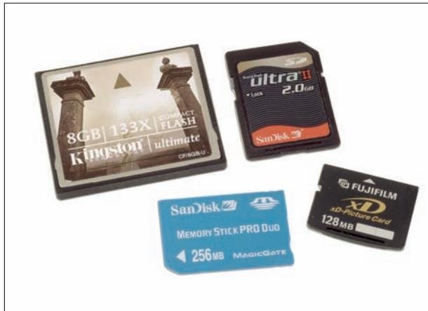
**Figure 2-3:** Clockwise from top left: CompactFlash, Secure Digital, xD, and Sony Memory Stick Pro Duo.
