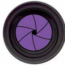
**Figure 1-9:** Lens opening, f-stop, aperture — all mean the doorway that light passes through to the sensor.
