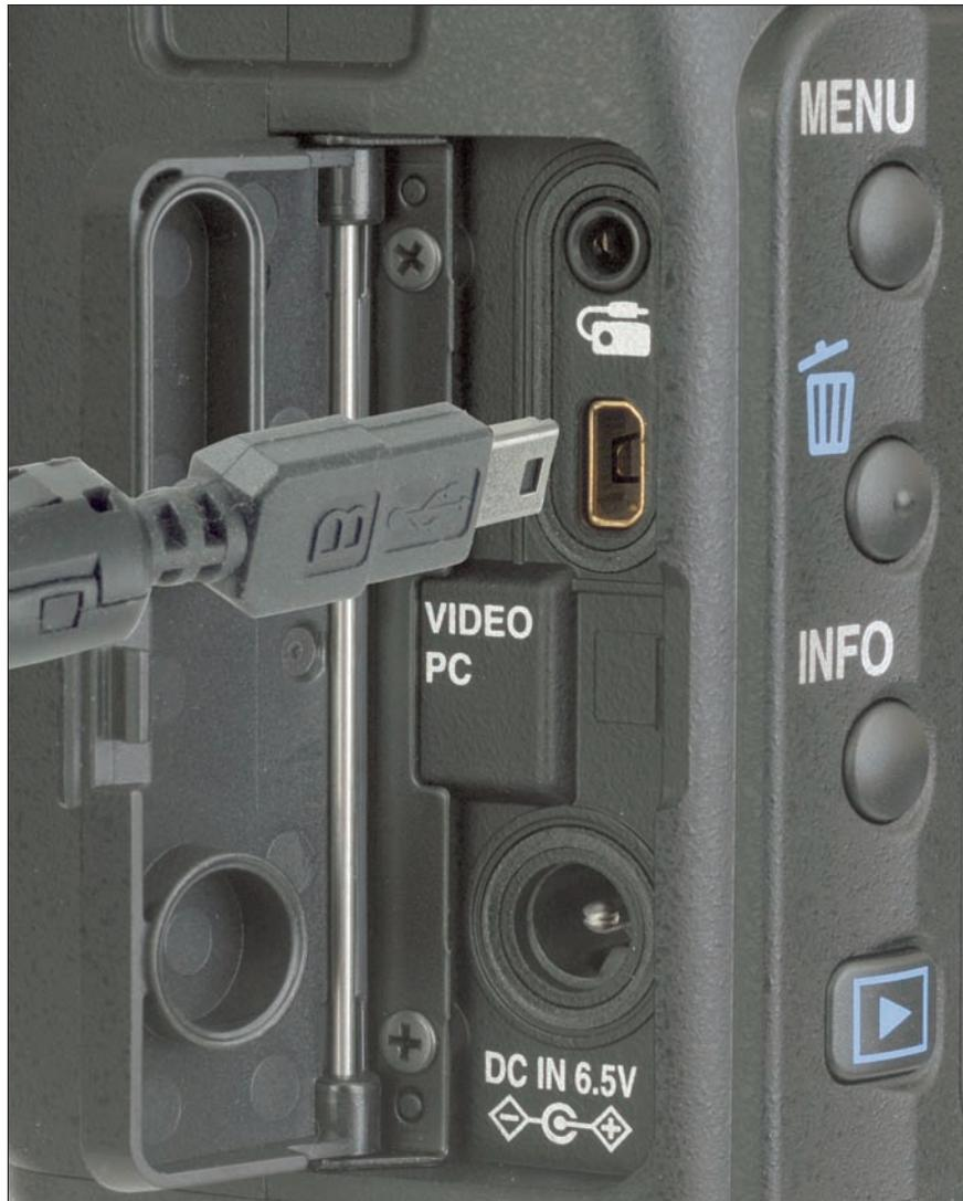
**Figure 2-1:** A USB cable can be plugged into your camera to link it with your computer.
