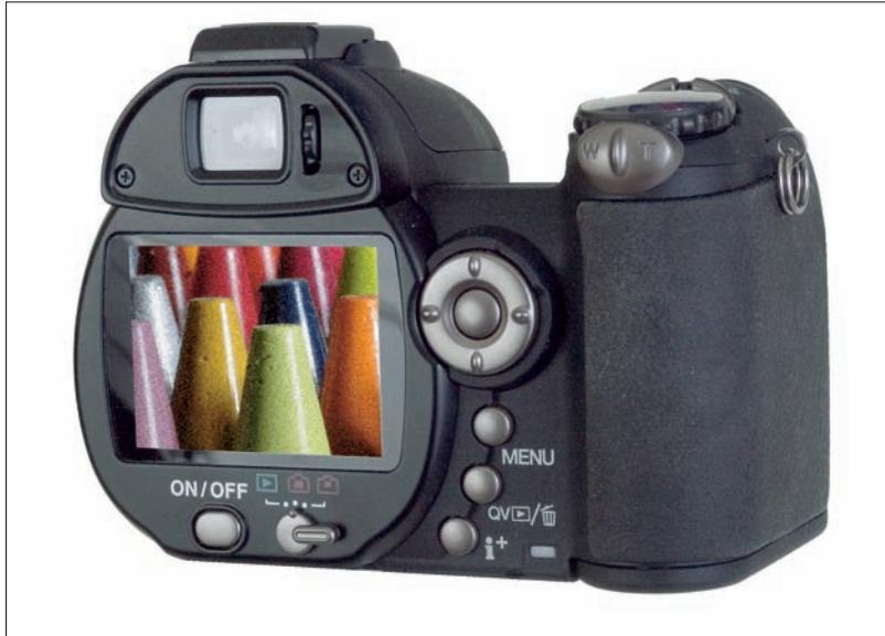
**Figure 1-3:** Advanced consumer models may offer both a back-panel LCD and a second EVF display seen through a viewing window.
