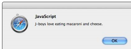
Figure 1-2: This message box is displayed from a JavaScript command inside the onclick handler.
