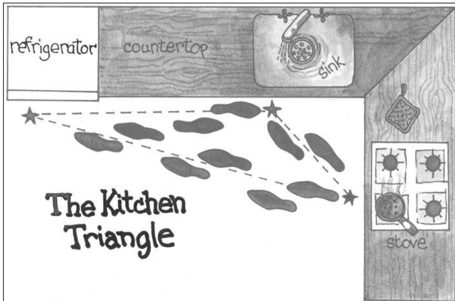
Figure 1-1: One example of an efficient kitchen triangle.
