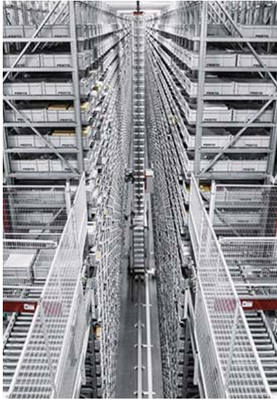
The automated warehouse system enables the processing of large order volumes. With storage capacity of 65,000 bins and the high performance picking and packing stations the system enables Festo to pick and pack more than 1,000 items per hour. (Photo: Festo)
