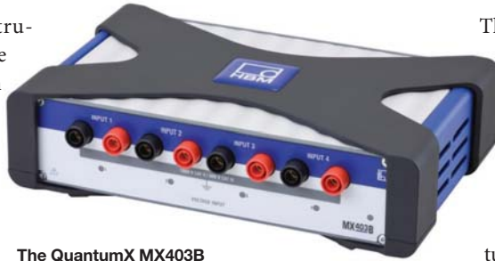
The QuantumX MX403B data-acquisition amplifier can measure low or high voltages at high electrical potential with CAT II or CAT III safety rating. This reduces the risks of working in high-voltage domains.
