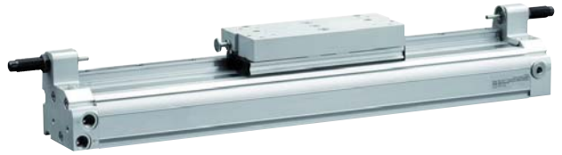
Rodless actuators offer the benefits of reduced weight and a smaller profile. They also have the ability to counteract offset loads.
