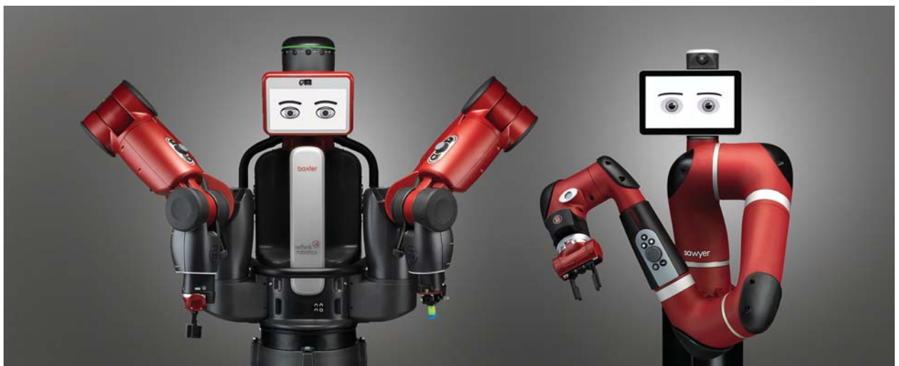
Baxter and Sawyer are the friendly collaborative robots, or cobots, from Rethink Robotics. They not only perform physical tasks, but are self-learning and continuous improvement equipment for the manufacturing line. (Image courtesy of the Rethink Robotics Inc.)
