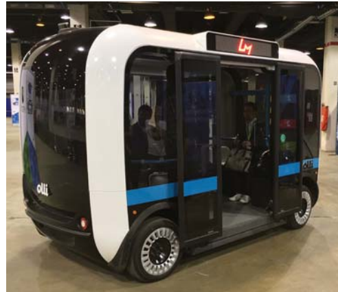
Olli is made of an aluminum chassis with carbon-fiber body panels, along with several 3D-printed parts, including the wheel wells, fenders, and interior kick panels.
