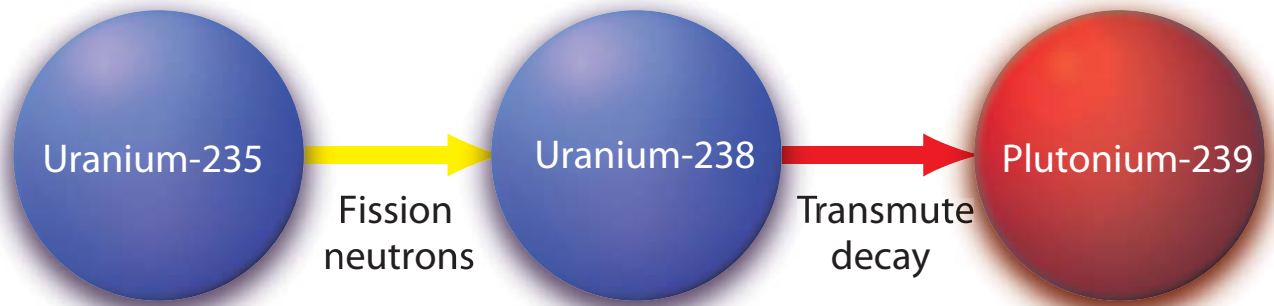
Uranium-fueled reactors consume uranium-235 and produce plutonium-239.
