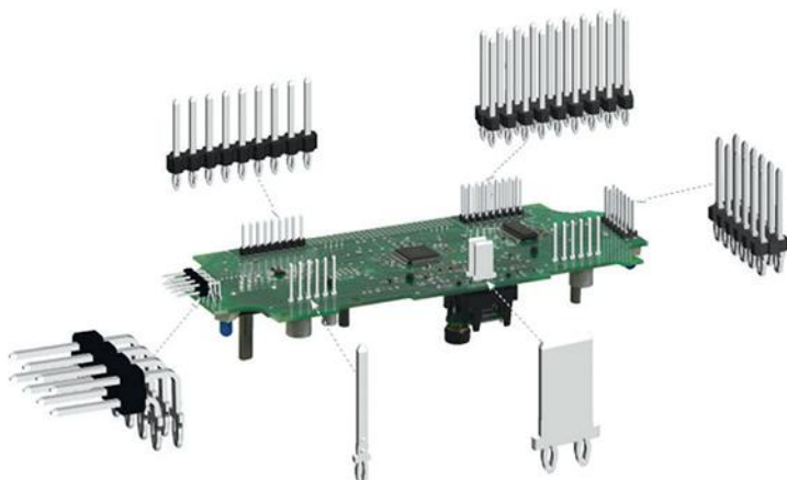
The Compliant technology developed by AutosplICE allows for friction-fit mating of interconnects, eliminating the soldering process. (Courtesy of AutosplICE)
