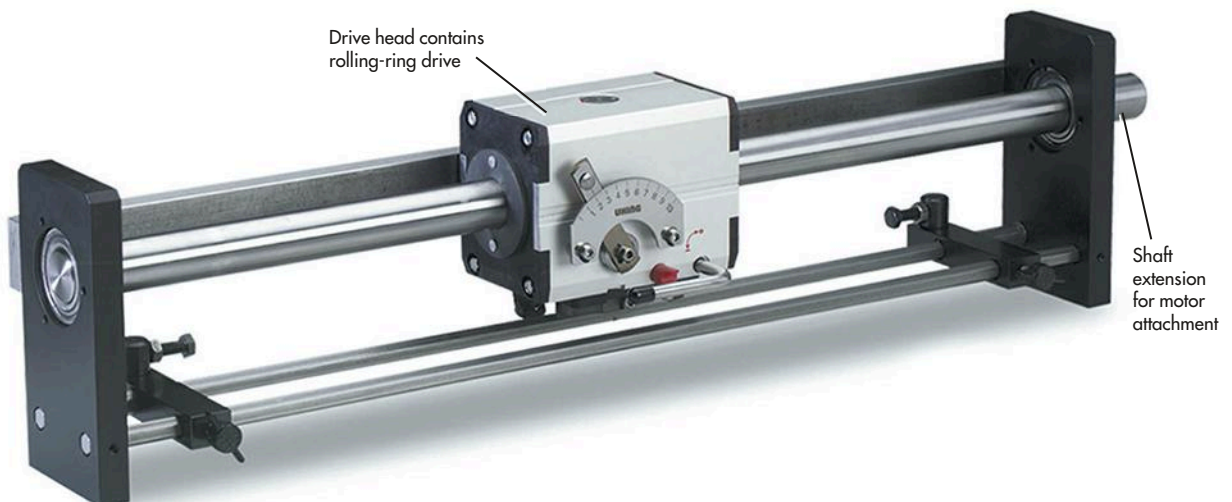
The rolling ring-drive housed in the drive head converts rotary motion of the shaft to linear motion for the drive head. In a packaging device, the head might hold a blade for cutting boxes or an adhesive applicator for laying down a bead of glue.
