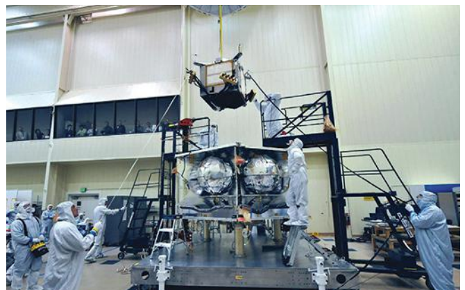
Technicians install the radiation vault around Juno's instruments in a Lockheed Martin clean room in Denver, May 2010. (Courtesy of NASA/JPL-Caltech/LMSS)
