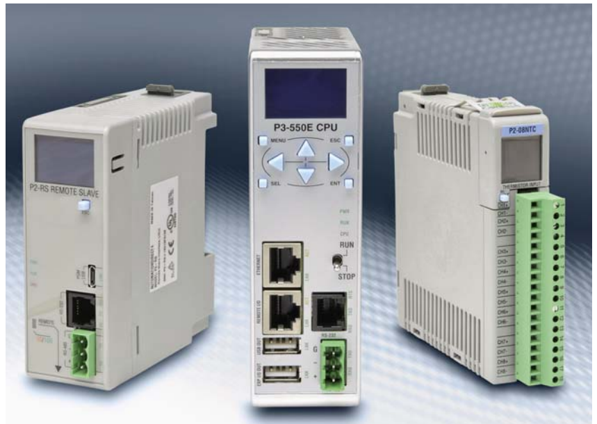
USB and Ethernet ports are standard on most current PLCs to improve connectivity, and help expand memory. The P3-550E high-performance CPU has multiple communications ports, including two USB and Ethernet ports, and one each for RS-232 and RS-485. The system is expandable with the P3-RS, P3-RX, or P3-EX modules. It also offers local, expansion, and remote I/O.
