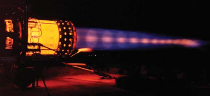
This image shows a Pratt & Whitney J58 on full afterburner. Shock diamonds appear in the plume of the engine. These are a formation of standing wave patterns caused by changes in density and pressure brought upon by shock waves.
