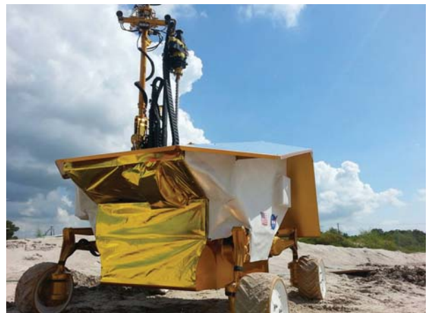
The Resource Prospector incorporates a solar-tracking solar panel to boost and store energy when in sunlight.
