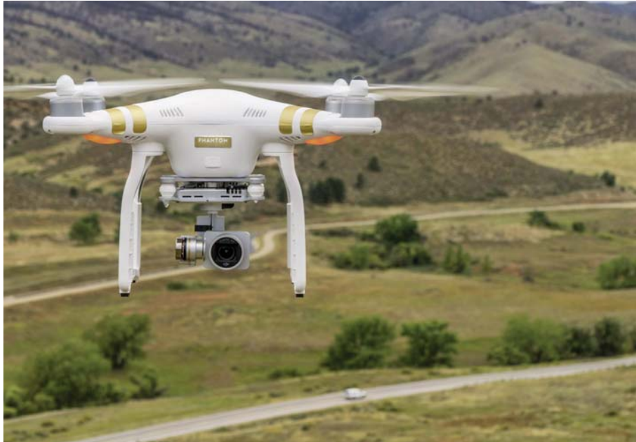
The Phantom 3 quadcopter from DJI lists for about $800, but can be found online for just under $500. It weighs almost 3 lb, can climb at about 16.5 fps and descend at 10 fps, and has a top speed of practically 36 mph. It can climb to 19,690 ft. above sea level, but it is usually set to a default of 400 ft. to stay within FAA guidelines.
