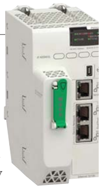
The new Modicon M580 from Schneider Electric is an Ethernet Programmable Automation Controller (ePAC) that features redundant processors, native Ethernet, and cybersecurity embedded in its core.
