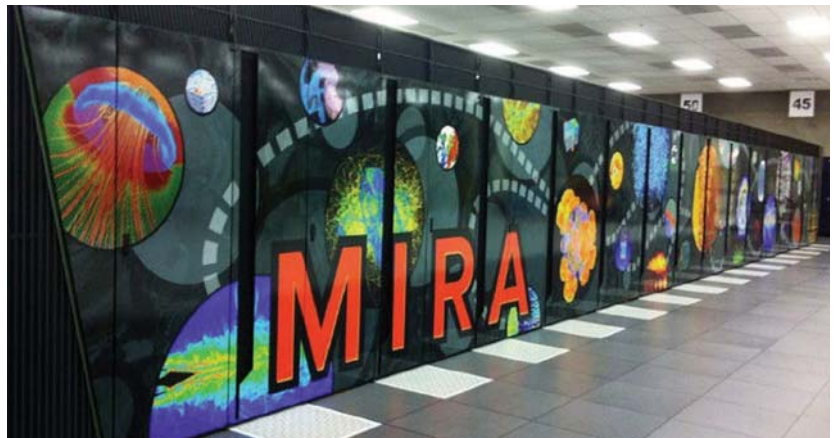
VERIFI uses the supercomputing power of IBM's Mira at the Argonne Leadership Computing Facility to simultaneously simulate thousands of complex engine-designs in as little as a few days. Mira consists of 48 racks and contains 768 terabytes of memory.
