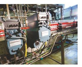
to reduce energy consumption by up to 50%, or more, compared to standard drive products. It is designed with high-efficiency individual components and combines the gearing, motor and drive electronics in a single unit. This makes it possible to do away with control cabinets, saving space, reducing costs and the time-consuming wiring of motors, sensors and actuators, not to mention the elimination of much of the costly cabling.
