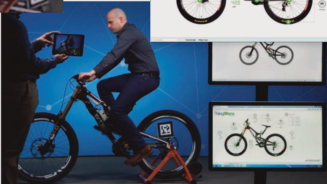
'Digital twin' brings together the digital and physical design worlds with augmented reality (left) showing real world data that can be harvested en masse, and utilised in the future to improve products
