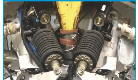
Carbon Spring system saves up to 70% weight
