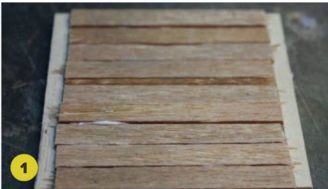
1 The five sides of the mould were made from wooden strips glued to a plywood base. The strips were then textured with a scribing tool and wire brush before being glued to the plywood.
