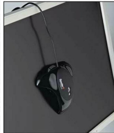
Turn the screen on, wait around half an hour for it to warm up and then let the Spyder4ELITE work.
