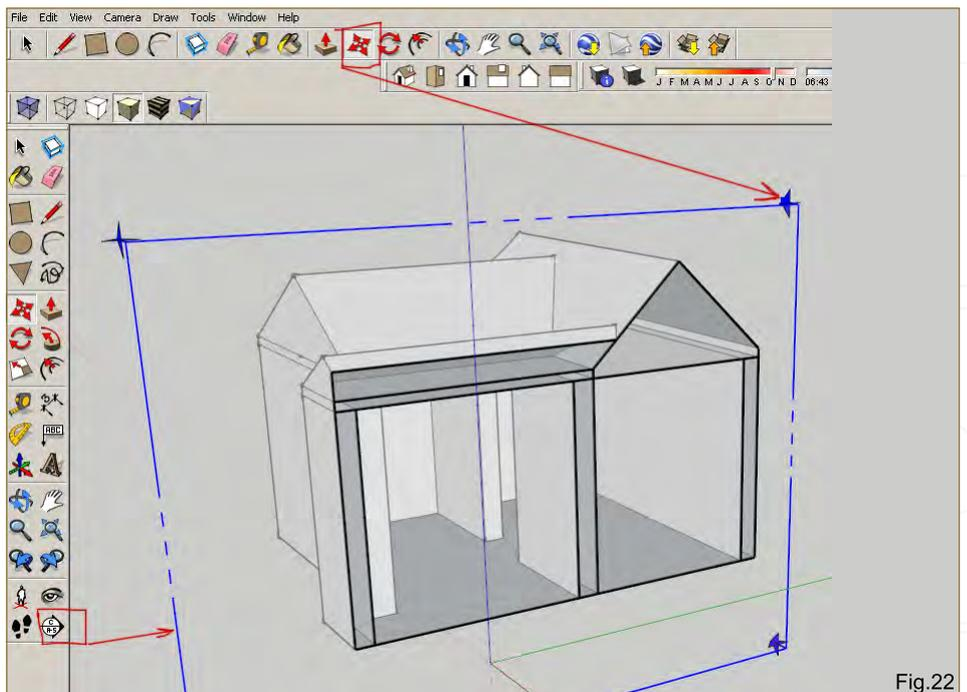
cross-section of your object. To use this click on the tool and then align the green icon to the corresponding plane or angle you wish to view. Then select the Move tool and click on one of the corner arrows and drag in the relevant direction (**Fig.22**).
