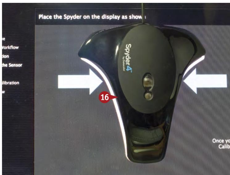
A window appears showing you where to place the sensor device on your monitor screen.
