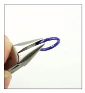
**8.** Now, bring your dominant hand forward, evening out the ends of the jump ring. Wiggle the ends into position by pushing and pulling the ends in tiny motions, so you get a seamless closure.
