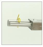
7. With your thumb, push the wire away from you and around the large barrel of the plier all the way around until it almost touches the loop.
