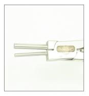
**6.** Flip the pliers over so now the 2mm barrel is facing you and the 4mm barrel is facing away from you.
