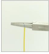
**3.** Place the wire between the jaws of the roundnose pliers at the mark that you made in step 2. Make sure the top of the wire is flush with the pliers.
