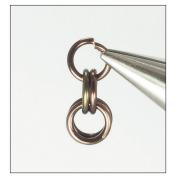
**4.** Take one open jump ring and scoop up the same two closed jump rings that you picked up in step 3. Close the jump ring.
