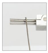
4. Holding the pliers in your dominant hand, place your other hand below the pliers and on the wire. Slowly bend the wire upward and around the 4mm jaw of the plier until the wire touches the point in between the pliers and slightly to the right of the end of the wire.
