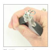
11. With your thumb, press the wire around the small 2mm barrel until the wire touches the cut ends and forms a closed circle. Release the wire from the jaws of the pliers.
