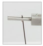
**5.** Relax the pliers and rotate the wire until the tail is below the plier's jaw, like it was in step 3.
