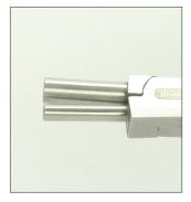
**5.** Hold the bail-making pliers so the small 5mm barrel is close to you and the large 8mm barrel is farther away from you.
