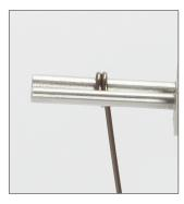
**7.** Relax the pliers and rotate the wire until the tail is below the plier's jaw, like it was in step 3.
