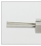
**2.** Hold the bail-making pliers parallel with the small barrel (2mm) facing you and the large barrel (4mm) facing away from you.
