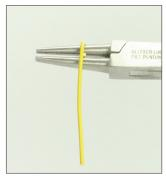
**4.** With your thumb, push the wire away from you around the jaw of the pliers all the way around until the wire touches the cut end on top, forming a closed loop.
