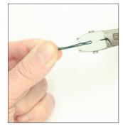
**3.** Use nylon-jaw pliers to get the bend at the top as close together as possible. Use little squeezes with the pliers to close. There will be a small space between the closure—that is perfectly OK.
