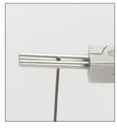
**3.** Grip one end of the wire between the pliers with the top of the wire flush with the top of the pliers.
