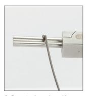
**6.** Re-grip the wire with the pliers, and with your non-dominant hand, bend the wire upward and to the right of the previous wrap. Bend the wire until it crosses the point in between the pliers.
