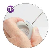
I leave the wire on the spool and extend it from the spool, straightening the wire by pressing it between nylon-jaw pliers before cutting it. That allows me to use the spool for leverage while I'm straightening the wire.
