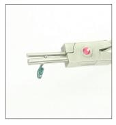
**10.** With the 4mm barrel facing you, insert the wire between the jaws with the bent portion of the clasp toward you and parallel to the barrels.
