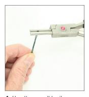
**4.** Use the small bailmaking pliers (the 4mm barrel should be facing you and the 2mm barrel should be facing away from you). Place the folded portion of the wire in between the jaws of the pliers, making sure the folded part of the wire is even with the barrels.
