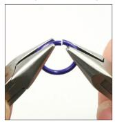
**5.** Place the split in the jump ring at the 12 o'clock position and place the tips of the pliers as close to the split in the jump ring as possible. Notice how close my hands are to the tips of the pliers?
