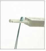
**7.** Place the wire between the jaws of the pliers with the hook portion of the wire facing you.
