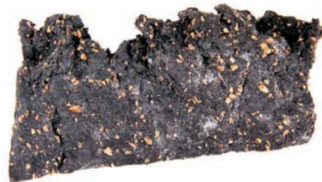
This material is a rubber and cork compound; it will be used to create rubber soles with cork pieces for texture.
