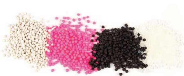
Balls of plastic as they look before being melted down to be used for soles.
