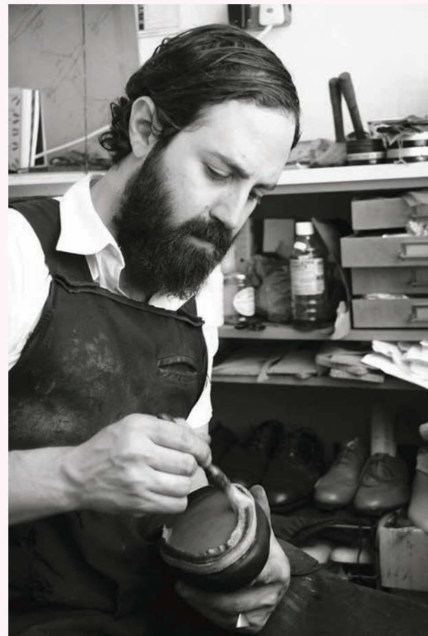
Sebastian applying adhesive to the bottom of the shoe; this preparation is only a fraction of the time-consuming process.
