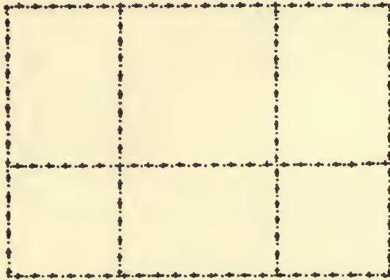
FIG. 79. ROOT TWO WITH TWO ROOT ONE'S OVERLAPPING MAKE THREE ROOT ONE'S AND THREE ROOT TWO'S IN SEQUENCE
