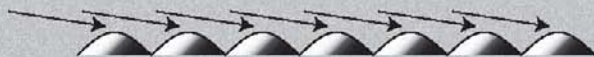
Light hits the surface at a shallow angle so that each peak casts a shadow in the next valley – micro contrast (texture).
