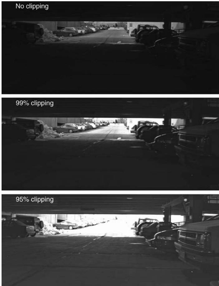
FIGURE 12.7 The choice of clipping the RGB image prior to display has a large influence on the final appearance of the rendered image. See color insert.
