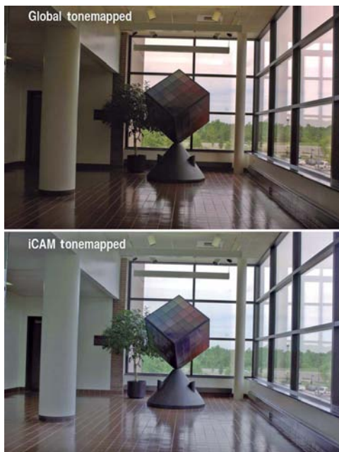
Figure 12.8 An example of a HDR image-rendered using the iCAM framework as described above.
