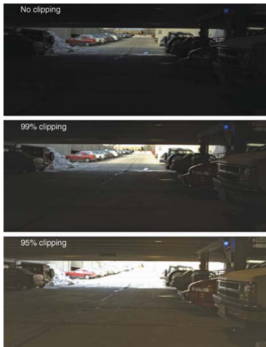
Figure 12.7 The choice of clipping the RGB image prior to display has a large influence on the final appearance of the rendered image.
