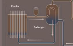
moderator, is pumped through the core of the reactor, and the temperature of the core increases by hundreds of degrees.
