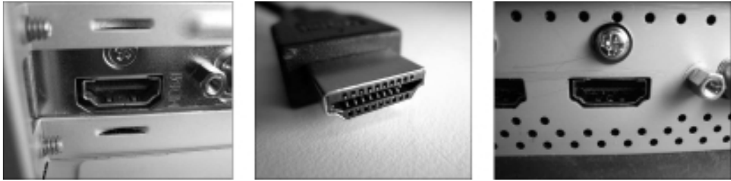
Figure 9-5: An HDMI port on a video card (left), cable connector (middle), and monitor (right).
