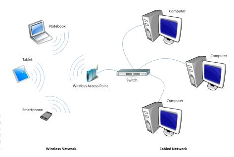
FIGURE 9-3: A wireless access point connects a wireless network to a cabled network.
