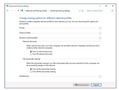
FIGURE 3-1: Enabling file and printer sharing.
