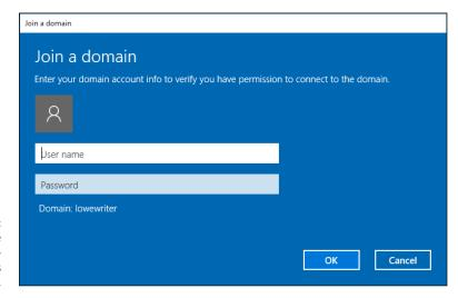
FIGURE 7-10: You must provide domain administrator credentials to join a domain.
