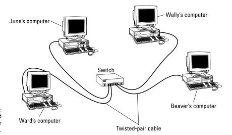
FIGURE 6-2: A network cabled with twisted-pair cable.
