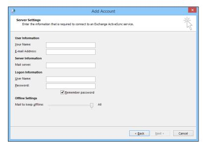
FIGURE 14-16: You must identify the Exchange server and provide a username.
