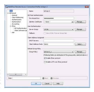
An IPSec configuration page on a Cisco ASA security appliance.
