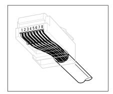
FIGURE 6-3: Attaching an RJ-45 connector to twisted-pair cable.
