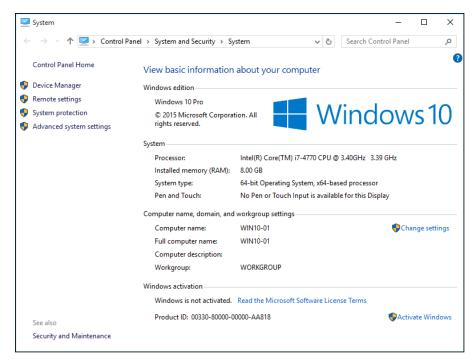
FIGURE 4-2: The Properties page for a computer with 8GB of RAM.
