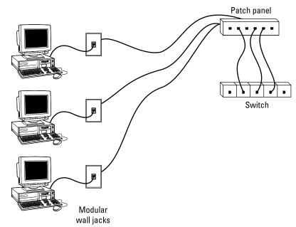
FIGURE 6-4: Using wall jacks and patch panels.
