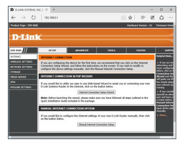
FIGURE 9-5: The main configuration page for a typical wireless router.
