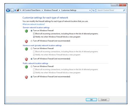
FIGURE 8-2: Activating the Windows firewall.
