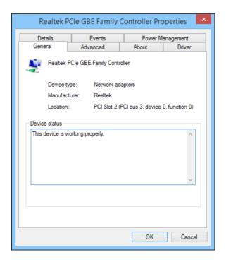
FIGURE 7-6: The Properties dialog box for a network adapter.
