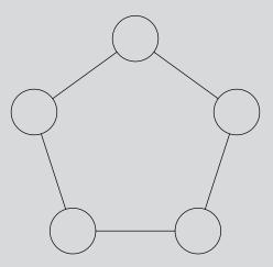
A ring is very much like a bus except with no end to the line: The last node on the line is connected to the first node, forming an endless loop.
