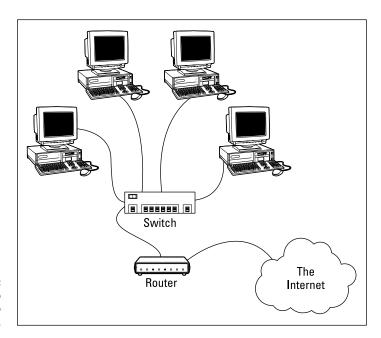
FIGURE 6-6: Using a router to connect a LAN to the Internet.
