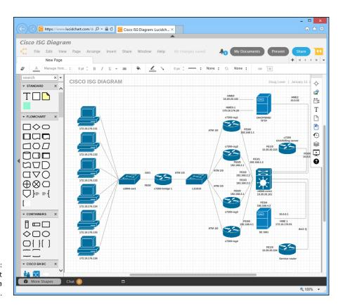
FIGURE 4-4: Using Lucidchart to draw a network diagram.
