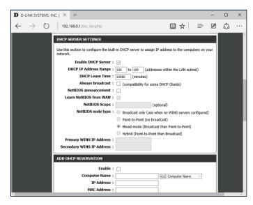
FIGURE 9-6: Configuring DHCP for a typical wireless router. Larger networks with more demanding DHCP requirements are likely to have a separate DHCP server running on another computer. In that case, you can defer to the existing server by disabling the DHCP server in the access point.
