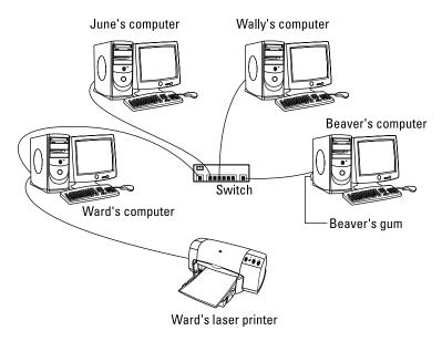
**FIGURE 1-1:** A typical network.
