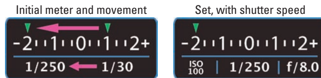
Figure 5-8: Move the exposure from the first reading to -2.0 EV to set your first bracket.
