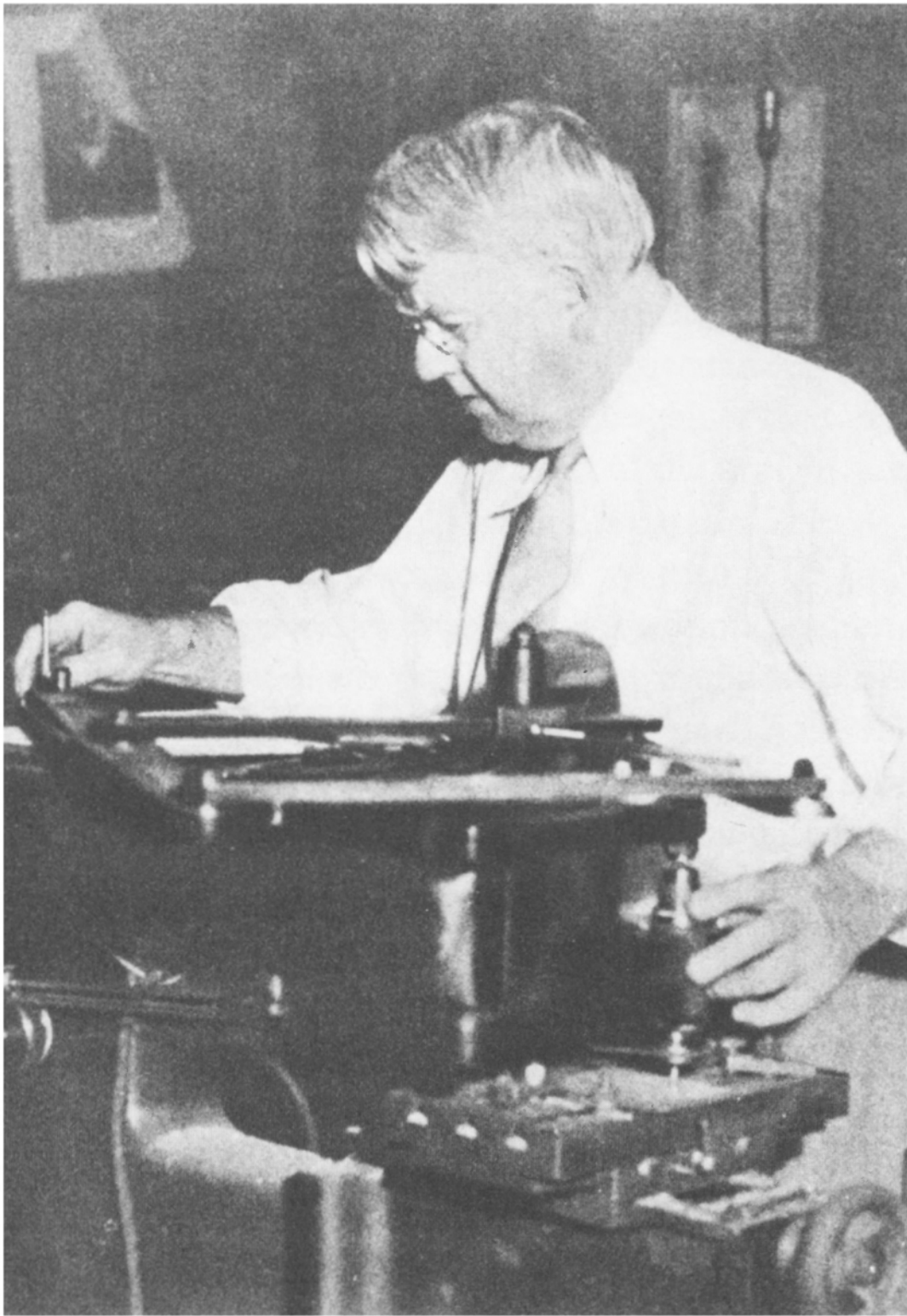
ENGRAVING THE WORK PATTERN IN METAL FROM THE MASTER PATTERN
